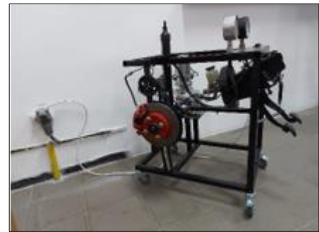
Figure 6. Experimental installation for intensive braking
